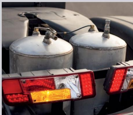
**Above:** The cooling system for the brakes gets pneumatic assist this year, the tanks for which sit at the back.
